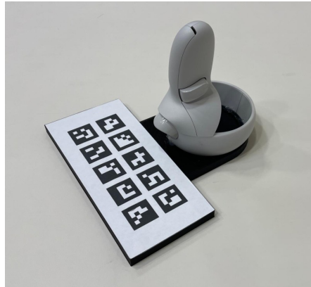
Figure 9. Calibration tool used to align coordinate frames between the RGB camera and the Meta Quest 2 headset. The controller is rigidly connected to the ArUco board.
